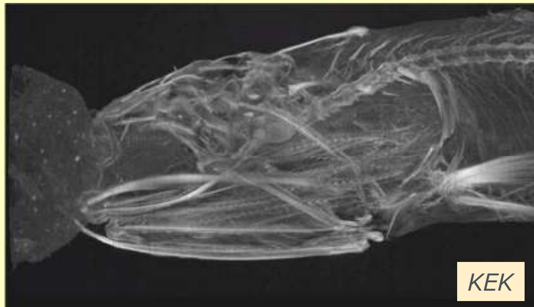
An example of X-ray image (small fish) taken by the integration-type SOI sensor (INTPIX4).
